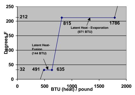
In the above graph, the amount of heat added to water is referenced from 0° Kelvin (absolute zero). The latent heat of fusion of water is 144 BTU per pound. In the process of freezing, water releases the same amount of heat (144 BTU / pound) that is absorbed in the process of melting.
